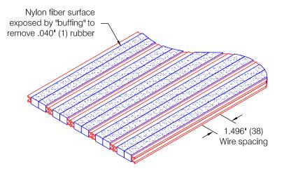
"CD": Closed Construction, Double Insert
