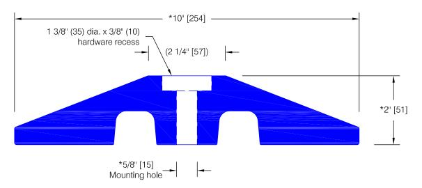
\* SBE-1025 is manufactured from recycled plastic. This product is subject to significant dimensional variation. End-to-end alignment is not guaranteed and should not be expected.
