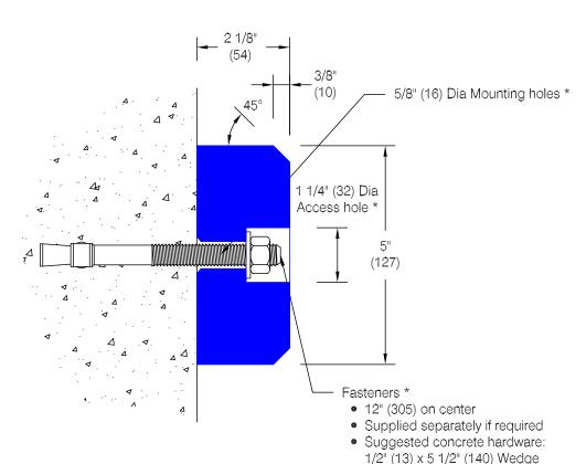
\* Standard bumper is supplied undrilled and with no mounting hardware. Hole spacing shown for bumpers 48" (1219) and longer. Contact factory for hole spacing on lengths shorter than 48" (1219).
