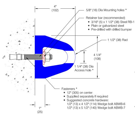
\* Standard bumper is supplied undrilled and with no
