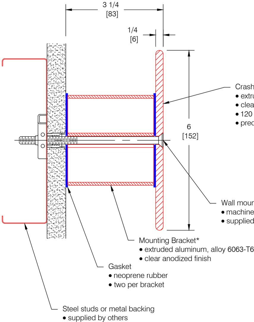
\* Nominal bracket spacing 32" on center. Actual bracket spacing will vary according to jobsite conditions. Maximum spacing not to exceed 48" (1219).
